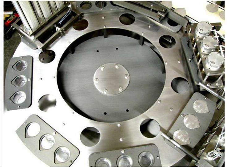
The cup seal position can be either **Die-Cut Foil** or **Roll Stock Film**. The die-cut foil station features a mechanically driven pick and place with a pneumatic seal head.
