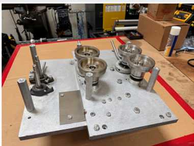
Fin Wheel Assembly After Refurb
